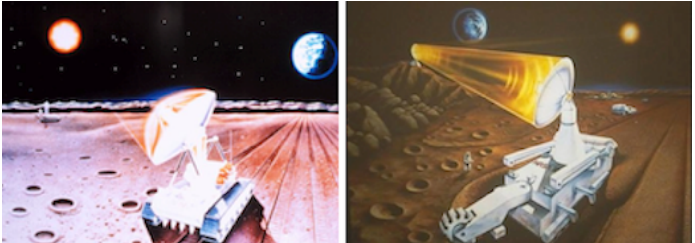
Two Helium-3 harvester concepts. One at right uses a static mirror to direct sunlight to the miner
