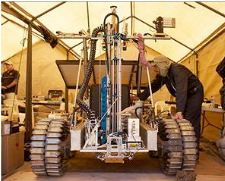
Canadian Space Agency (CSA)'s Artemis Jr. rover holds the Regolith and Environment Science and Oxygen and Lunar Volatiles Extraction (RESOLVE) instruments to drill for water ice and other resources during a simulated mission. Photo: NASA/Joe Bibby
